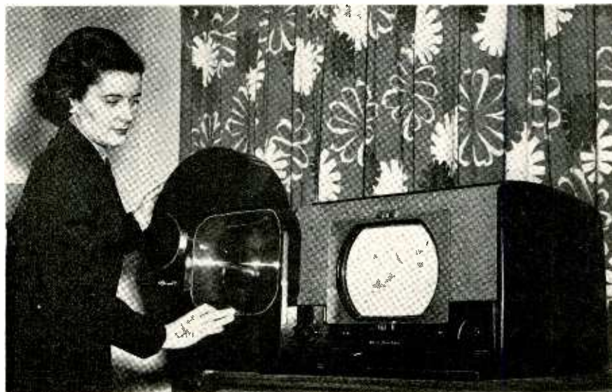
10-inch TV set with removable 22½-inch color converter. See text for explanation.
